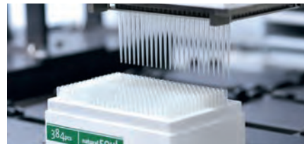
Multiple Channel Arm picking up one row of 24 50 \mu\text{L} tips
