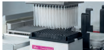
Multiple Channel Arm picking up 96 500 \mu\text{L} disposable tips
