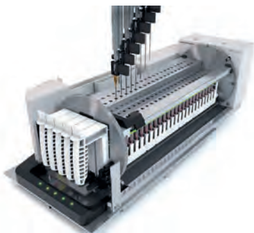
Sample mixing and aliquoting with the Fluent Mix and Pierce Workstation
